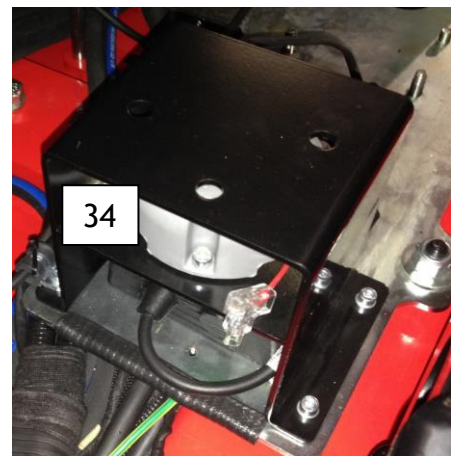
36. Endschalter "Proactive leveling"
